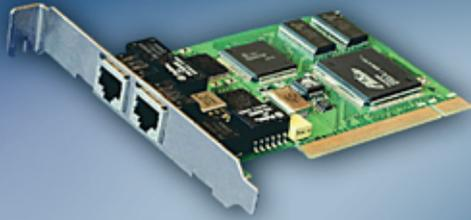
PCI card Tahoe 931 and Tahoe 932 cards are equipped with, respectively, one and two V.35 interfaces. They may work in both unframed or framed mode.
