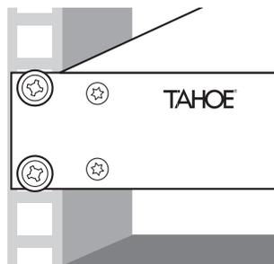
1. Position the device in the rack and align the holes in the mounting brackets with the holes in the rack.
